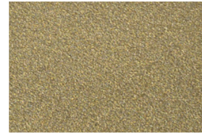
RAL 1035 Pearl beige / Perlbeige 97.50 % powder coating / Pulverlack RAL 7006 fine texture / Feinstruktur 1.50 % SYMIC PCE C001 1.00 % SYMIC PCE C393
