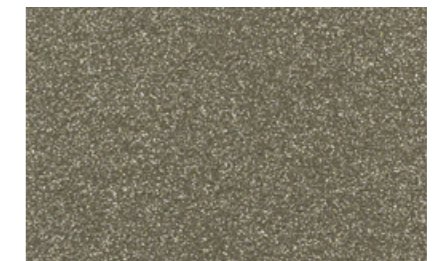
RAL 9007 Grey aluminium / Graualuminium 95.00 % powder coating / Pulverlack RAL 7039 fine texture / Feinstruktur 2.50 % STANDART® PCBF 3500 2.50 % STANDART® PCBF 5000
