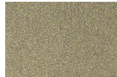
RAL 7048 Pearl mouse grey / Perlmausgrau 97.50 % powder coating / Pulverlack RAL 7039 fine texture / Feinstruktur 1.65 % SYMIC PCE C001 0.75 % SYMIC PCE C393 0.10 % SYMIC PCE C522
