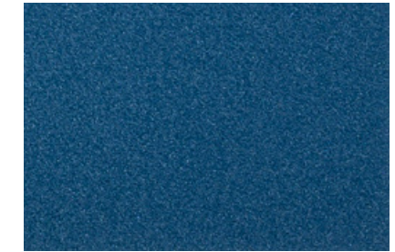
± DB 510 99.40 % Pulverlack / powder coating RAL5001 Feinstruktur / fine texture 0.40 % SYMIC PCE A001 0.20 % SYMIC PCE C001
