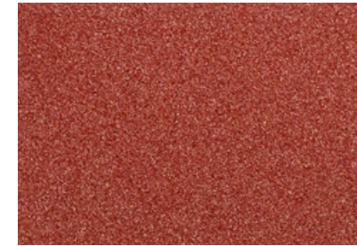
± DB 301 97.50 % Pulverlack / powder coating RAL3011 Feinstruktur / fine texture 2.00 % STAY/STEEL LN 25 0.50 % SYMIC PCE A001
