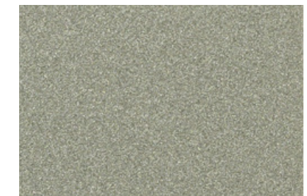
± DB 704 96.00 % Pulverlack / powder coating RAL7023 Feinstruktur / fine texture 2.00 % STAY/STEEL LN 25 1.00 % SYMIC PCE A001 1.00 % SYMIC PCE C001
