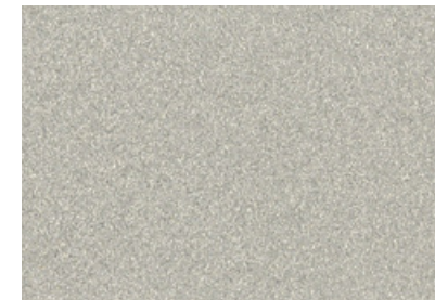
± DB 701 96.00 % Pulverlack / powder coating RAL7004 Feinstruktur / fine texture 2.00 % STAY/STEEL LN 25 2.00 % STAY/STEEL LN 35
