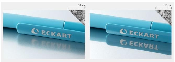
The original object, which is reflected in a transparent plastic substrate coated with a standard VMP (left) and METALURE® C - series (right). The C series shows significantly higher clarity of image compared to the standard VMP.
