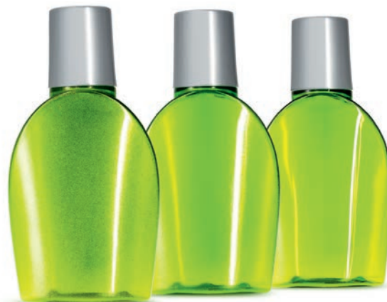
Fig. 4. Transparency in various facets with glass-based effect pigments: Platalux pigments create a translucent glitter appearance (left) and Luxan pigments create brilliant effects (center). For comparison: a plastic without effect pigments (right)
