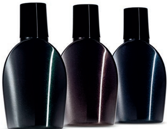
Fig. 3. Black isn't always black: with "colorful" Luxan pigments, various shades of color ranging from green (left) to red (center) or blue (right) can be created in dark plastics
