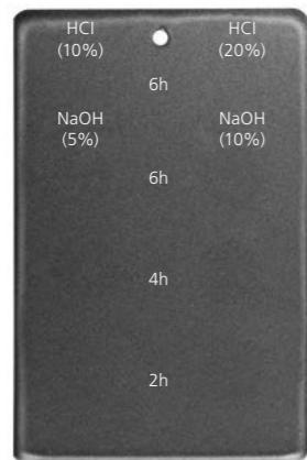
Corrosive reagents are dropped onto a powder coated test panel:
