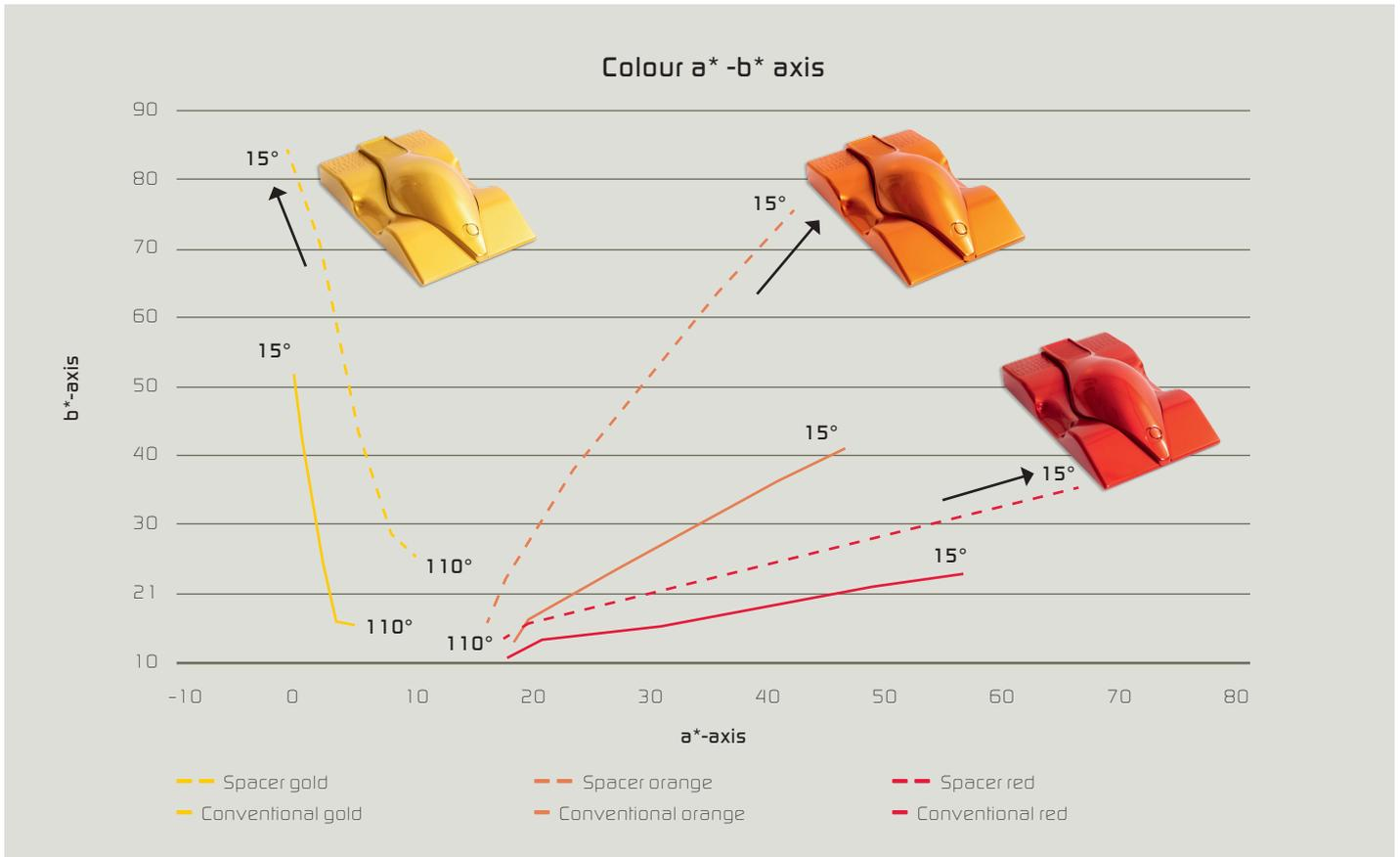
Figure 6: Colour and effect measurement via BYK mac, colour intensity C\*15 and sparkle intensity Si15.
